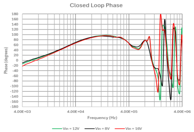
Figure 14. Closed Loop Phase (IOUT = 40 A)
